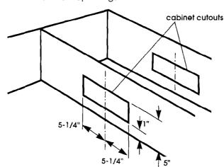
To vent through the roof with 3-1/4" x 10" rectangular ductwork, mark a line 1" and 5" from the back wall on the underside of the cabinet. Mark lines 5-1/4" to the right and left of the centerline on the underside of cabinet that connect the lines just drawn. Use a saber saw to cut a rectangular opening for the ductwork. Repeat for the underside of the top of the cabinet.
